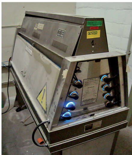
Figure 4. QUV testing equipment
