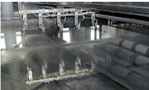
Figure 2. Application of the Ag to the glass
