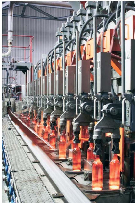
AIS 12 Section 6 1/4" DG, Servo Extraction. © Emhart Glass
