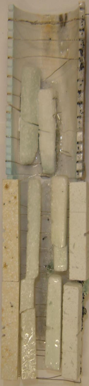
Typical result: Silica corrosion
